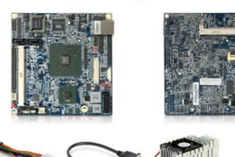
The VIA EPIA NR Nano-ITX embedded board is powered by the 1GHz VIA C7® processor, enabling convection cooled systems in locations where noiseless or dust-free systems are essential yet providing desktop performance with a maximum CPU TDP of just 9 watts and average operating power of well below 1 watt.
